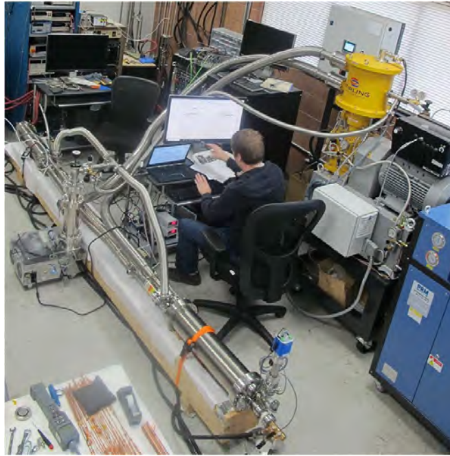
Figure 32. 20–30 K cooling loop set-up to cool DC cables. Courtesy of Advanced Conductor Technologies LLC, Boulder CO, USA
