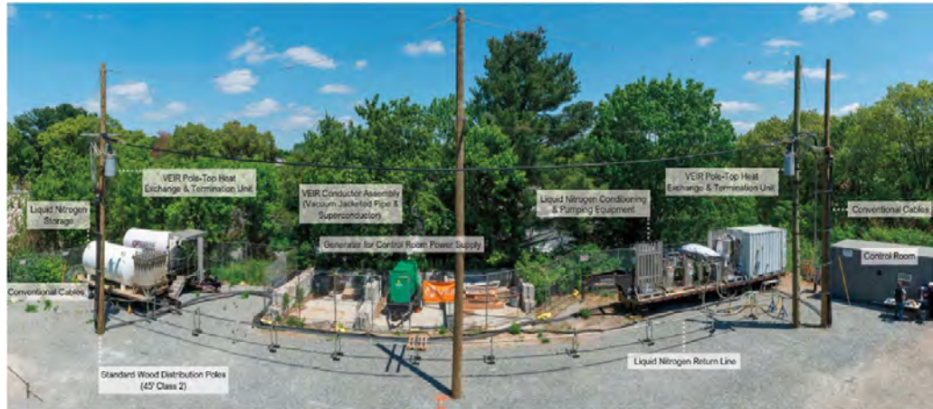
Figure 14. Shows a 30 m single-span suspended version of the O-SCTL demonstrated to understand withstand against outdoor environmental conditions and to utilize commercially available power line structures.
