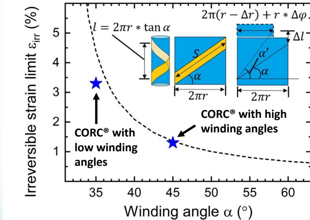
Enhanced critical axial tensile strain limit of CORC<sup>®</sup> wires: FEM and analytical modeling, V.A. Anvar, K. Wang, J.D. Weiss, K. Radcliff, D.C. van der Laan, M.S.A. Hossain, A. Nijhuis, *Supercond. Sci. Technol.* **35**, 055002 (2022)
