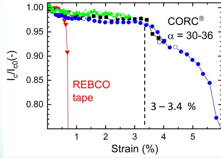
**Tape winding angle drives the irreversible strain limit in CORC<sup>®</sup> wires**
