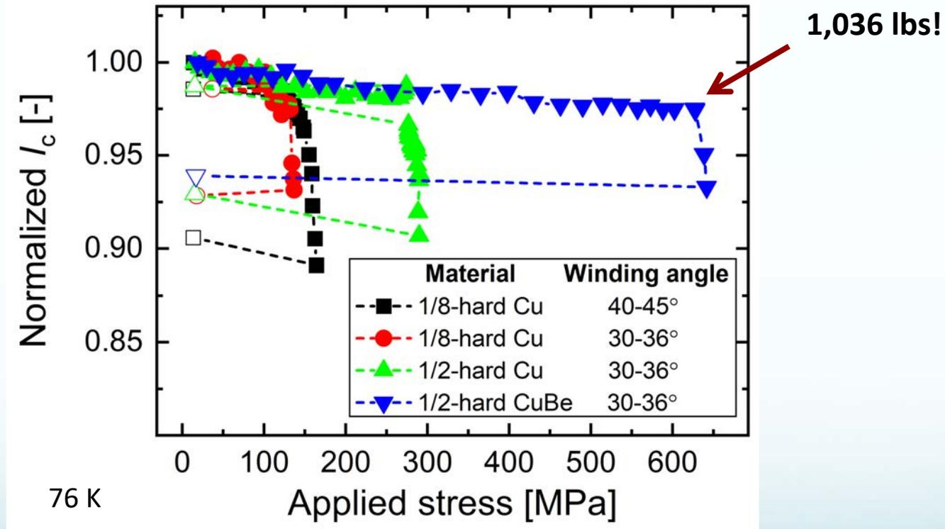
Irreversible tensile stress limit of CORC<sup>®</sup> wires can be engineered to exceed 600 MPa at 77 K
