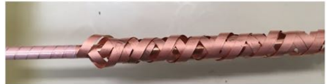
Figure 3. End of CORC ® wire with polyester heat shrink tube partly removed to show tapes springing apart from former.
