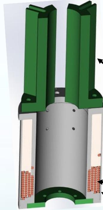
CORC<sup>®</sup> S-Bend through G10 slots utilizes CORC<sup>®</sup> flexibility to allow vertical travel of insert due to CTE mismatch between probe/coil-insert and LTS magnet
