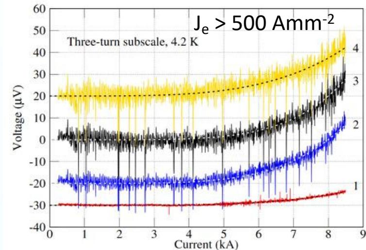
Feather M2 HTS dipole magnet demonstrator (18.5 m Roebel cable)
