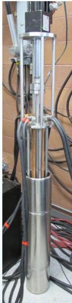
High-current tensile tests performed in liquid nitrogen
