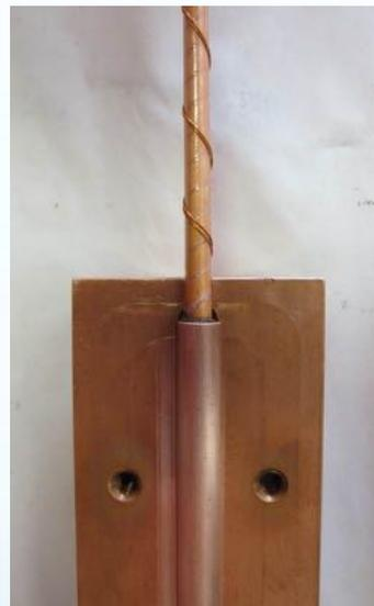
Critical stress significantly increased by using stronger former material
