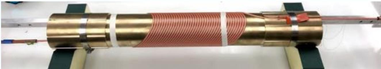
Xiaorong Wang: See talk Wk1L0r4B-02 - Development of Canted-Cos $\theta$  dipole magnets using CORC<sup>®</sup> wires
