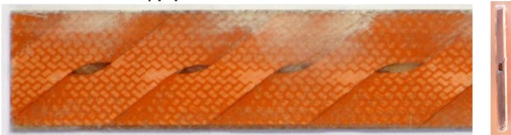
**Figure 4.** The structure of the impregnated Roebel cable.
