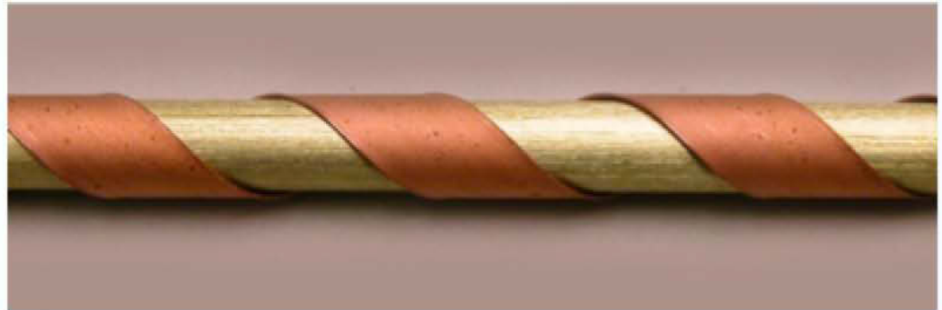
Single tape wound into a CORC® cable
