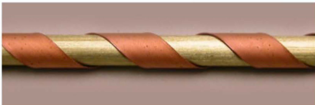
Single tape wound into a CORC® cable
